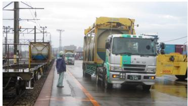
In Kanazawa, Japan they were able to see the LNG containers being offloaded to be drayed. At the destination LNG was pumped out into storage tanks for residential and commercial use. The company representatives were very helpful and the research team was impressed with the efficiency of the LNG container system and the impeccable safety record over 15 years of operation. A full report will be available in the fall of 2015
