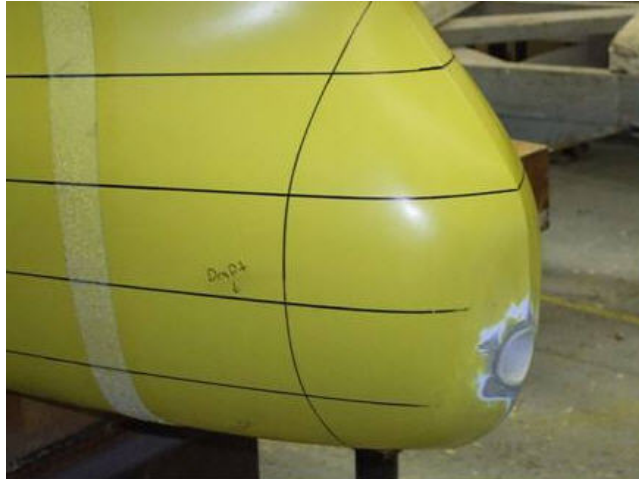
Figure 3.3: Location of Forward Ballast Trunk Inlet
