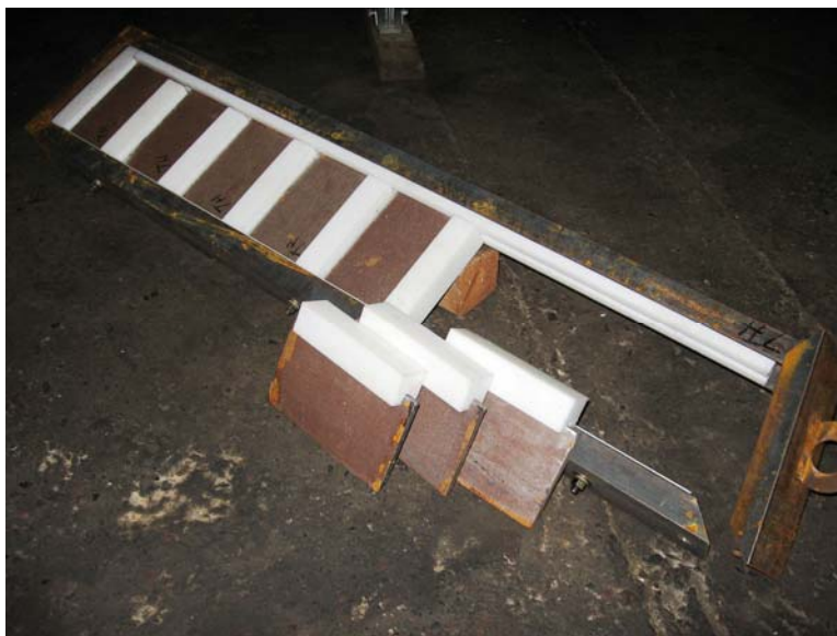
Figure 2. Photograph of metal tray frame and sheet steel coupons (separated by white HDPE spacers) before being installed in the Duluth-Superior Harbor during October 2006. [Photograph courtesy of AMI Consulting Engineers]
