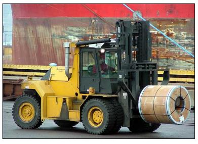
forklifts with diesel oxidation catalysts (DOCs). The DOCs are designed to reduce diesel pollution through a retrofit of the diesel exhaust systems. The DOCs are expected to reduce vehicle hydrocarbon emissions by 50%, monoxide emissions by 40% and particulate matter emissions by 20%.
