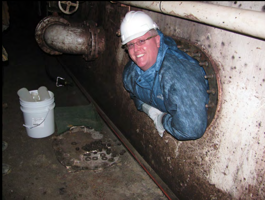
Sampling sediment from ballast tank of American Century. Photo credit: Carol Wolosz
